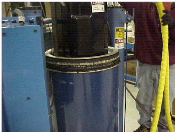
5. Make sure seal clears top of drum position
