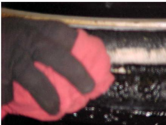
9. Grease seals (use proper grease)
